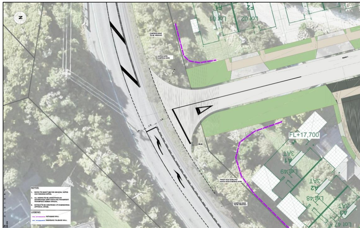
Figure 24: Indicative Works for Access
